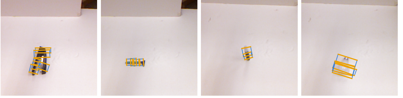
Fig. 2. Cornell Grasping Dataset samples after the evaluation transform ( 350 \times 350 center crop resized to 224 \times 224 ), with ground-truth grasp rectangles overlaid: jaw-opening edges in yellow, plate edges in blue.
